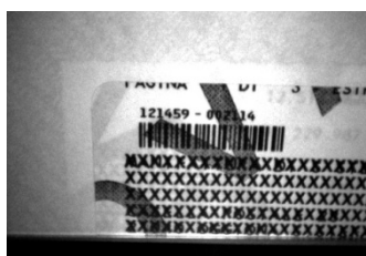
Figure 21 - Overprinted Barcode Readable by Matrix 320 also Through the Envelope Window Film
